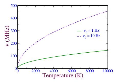
Figure 1: Variation of emission frequency ( $\nu$ ) with heating temperature (T)
