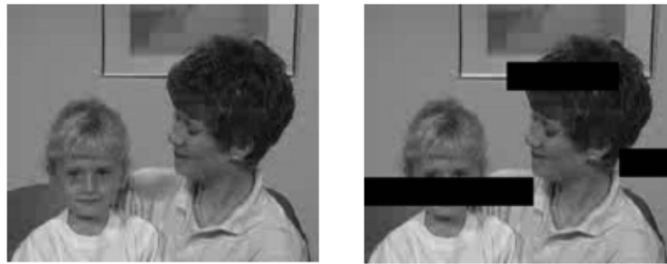
Fig. 3. (a) Decoded 8-th frame; and (b) Missing macro block location for the Mother and Daughter sequence (inter frame).
