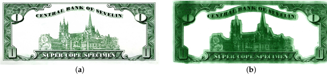
Figure 3. Effect of wiping errors in the intaglio printing process [92]. (a) Error-free intaglio print result; (b) Print errors caused by wiping errors.
