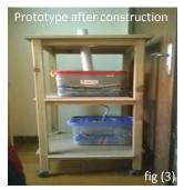
end, a wooden stand was constructed to provide a stand that can carry the whole system as shown in (fig.3)
