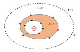
**Figure2.** A closed surface S enclosing the whole conductor. The net electric flux through the closed surface is zero, due to the electric field is zero everywhere outside the conductor.
