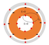
**Figure5.** A spherical electric charge layer encloses a conductor cavity. A closed surface S contains two parts. One part is in the cavity and the other inside the body of the conductor.
