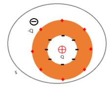
**Figure4.** A neutral conductor cavity enclosing a positive electric charge Q and there is another negative electric charge -Q in the vicinity of the conductor. S is a closed surface enclosing the whole sytem.
