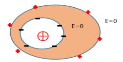
**Figure1.** A nuetral conductor cavity containing a positive electric charge. Under electrostatic equilibrium state, the electric field is zero inside the body area of the conductor and in the area outside the conductor.
