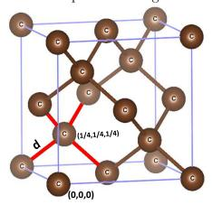
Carbon atoms in diamonds are arranged in a strong tetrahedral structure. The unit cell of a diamond is shown in the figure at left. Here  $a_o$  is the cubic lattice constant and d is the C-C bond length of 0.154nm. The four thick lines represent a tetrahedral geometry. The small size of a carbon atom and the tight covalent bond of carbon atoms in diamond structures are responsible for almost all of its unique mechanical, chemical and electronic properties.
