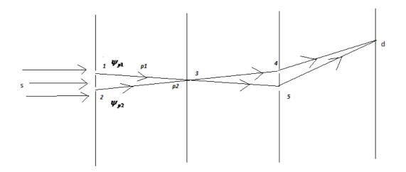
**Fig 1.** The modified double slit apparatus, p1 and p2 shows the possible paths for the photon to reach detector d. At hole 3 we have a minima and in the path p1 the photon leaves from slit 1 goes through slit 5 and reaches d and in path p2 the photon leaves from slit 2 goes through slit 4 to reach d.
