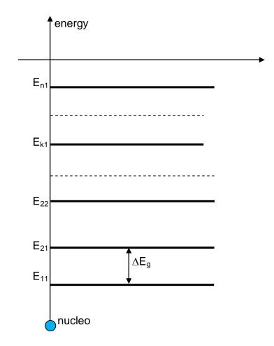
Fig.4 Discrete distribution of energy levels in one atom in which  $\Delta E_g$  represents the spectral gap
