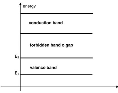
Fig.5 Energy bands in a non-conductor and in a semiconductor
