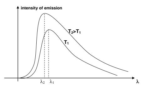
Fig. 3 Emission spectrum of black body for two different temperatures in function of wavelength
