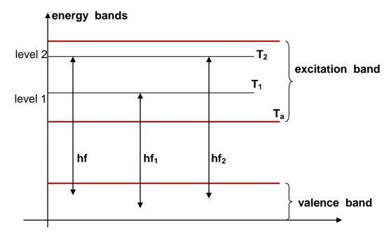
Fig. 2 Energy bands and energy quanta in the condensed matter
