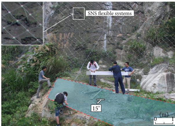
FIGURE 5: Photograph showing the fractured rock mass and the measurement area of rock joint set.
