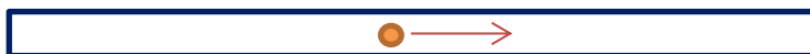
Figure 1. A particle moves back and forth in a tube, which works like a simple mechanical clock.
