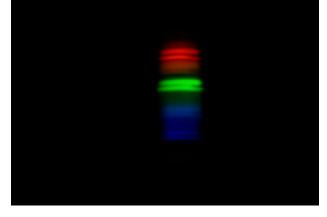
The amplitude of the wave increases the more the paper slit's angle decreases to the spectroscope slit. When the paper slit is parallel to the spectroscope slit, all emission lines have a line going through them. A larger angle to the spectroscope slit will produce a more squished spectral wave, until 90 degrees is reached, when the spectral wave straightens out into one continuous line.
