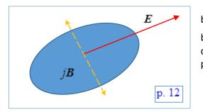
The vector E belongs to the plane defined by bivector jB. The area of the circle which presents the bivector is B, so its radius must be  $\sqrt{B / \pi} \approx 0.56 \sqrt{B}$ . The direction and possible orientations of the wave propagation are plotted in p. 12.
