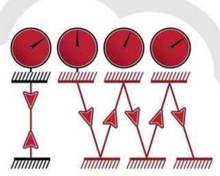
For this clock, each tick is the round trip of a light beam. If the clock moves, it takes longer to tick: Time slows down.
