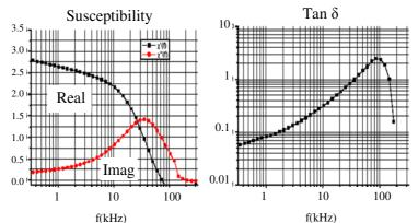
Figure 6 – Hysteresis loss in typical ferrofluid (Courtesy Sustech Gmbh)
