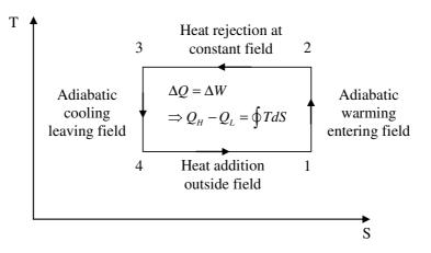
Figure 3 – T-S diagram MCE Carnot Refrigerator
