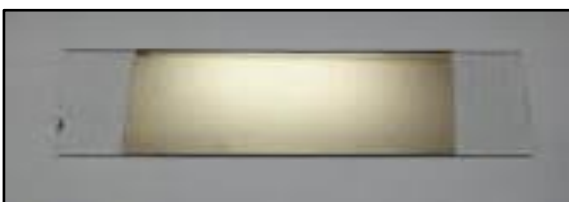
FIGURE 2 (a). Thin film coated Aranmula cast mirror without an image
