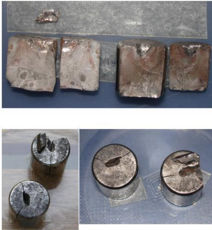
Fig.2b Two typical results of fusion ignition, wherein the local gas pressure has forced a wedge of steel downwards through the lower bearing, splitting it apart. One of the wedges is shown at top left, and sitting on the appropriate bearing in the lower views. It is triangular in cross-section, roughly 4mm x 1mm x 2mm deep.
