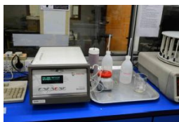
Anton Paar SVM 3000 Stabinger Viscometer
