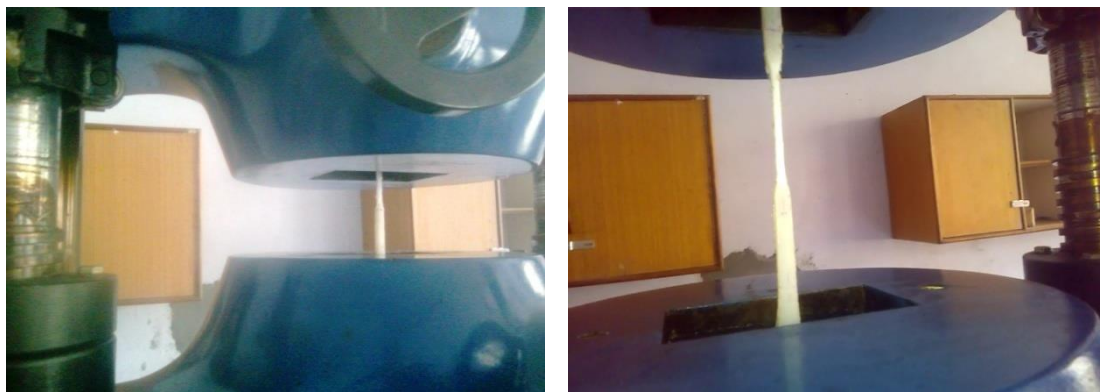
Figure 2:- Tensile Test of Nylon Fiber on Digital UTM
