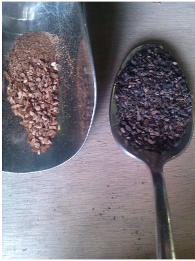
Figure 2: Photograph of original and torrefied hazelnut shell
