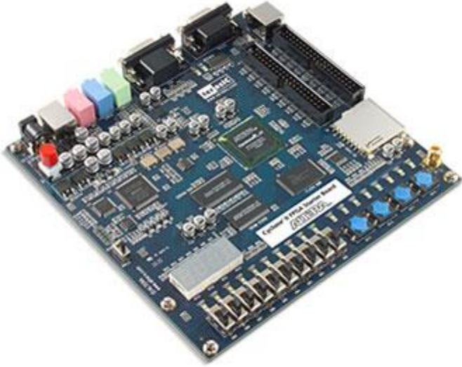
Fig. 4.1 Altera DE1 Board
