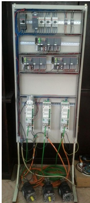
Figure 6.1 –The simulation bench for the control laws
