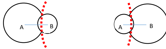
Fig. 3.1: The locus of the intersection points is depicted with red broken lines for both cases, when source A is stimulated before source B and vice versa.
