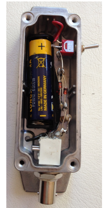
Fig. 1: Left: Circuit of Zener Diode Space Flow Detector, showing 1.5V AA battery, two 1N4728A zener diodes operating in reverse bias mode, and having a Zener voltage of 3.3V, and resistor R=10K\Omega . Voltage V across resistor is measured and used to determine the turbulent space flow driven fluctuating tunnelling current through the Zener diodes. Correlated currents from two collocated detectors are shown in Fig.4. Right: Photo of detector with 5 Zener diodes in parallel.
