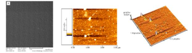
... The films are subsequently reduced to form nanoparticlat palladium film by increasing temperature ... The temperatures of annealing process were 450 degrees C
