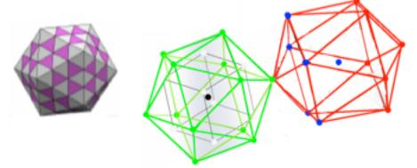
**The most stable** (lowest Energy per Atom) **Icosahedral Pd cluster is 147-atom**. Since the 147-atom Pd cluster has a metastable cuboctahedral state it can undergo the Jitterbug transformation that is necessary
