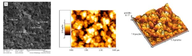
... SEM ... showed a grain structure ... size of grains ... 44 nm ... for 450 degrees C ... The Atomic Force Microscopy (AFM) images confirmed results ... that ... increasing ... temperature ... increases crystal structure ...".
