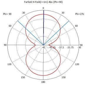
Fig. 4(b). H-field of proposed antenna
