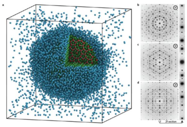
... Diiffraction reveals two-fold, three-fold and five-fold symmetry axes ... A detailed analysis reveals the absence of detectable phason strain ... which allows us ... to identify the solid as indistinguishable from an IQC ...
