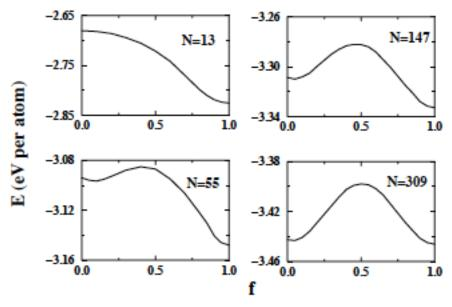
... f is a fraction of the displacements ... f = 0 and 1 correspond to the ... cuboctahedron and icosahedron, respectively ...".
