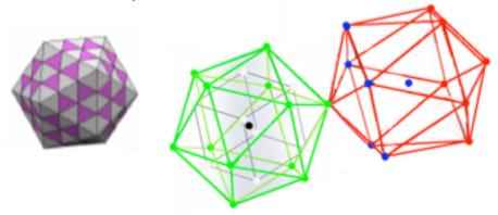
The 4-shell icosahedral structure contains 309 atoms (2.00 nm).
