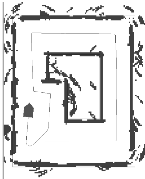
Figure 11: Map building based on the CFMW after improving the sonar model.
