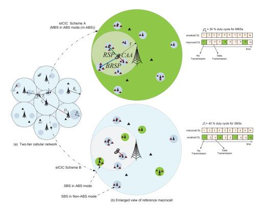
Fig. 1. (a) Graphical illustration of a two-tier smallcell network. In this part of the figure, the distances are demonstrated graphically. (b) Enlarged view of the reference macrocell illustrating eICIC scheme-A for MBS (when MBS is in ABS mode (m-ABS)) and eICIC scheme-B for SBS (when  $S'_1$  SBSs are in
