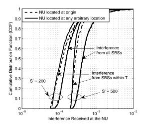
Fig. 5. Comparison of the CDF of the cumulative interference from S and S' SBSs considering (i) the exact location of the NU; (ii) NU is located at origin (assumption) (for T = 100,  $P_m = 10W$ ,  $P_s = 0.1W$ ,  $\beta = 2.0$ ).
