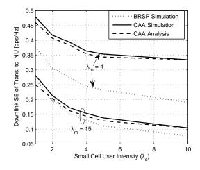
Fig. 8. Downlink SE of transmission to the NU with increase in smallcell user intensity ( $\lambda_s$ ) for different user association schemes (for  $\rho_m = \rho_s = 0$ ).
