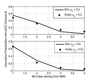
Fig. 6. Association probabilities of the NU with reference MBS and Q' active SBSs in eICIC scheme B (for  $R_m = 300 \text{ m}$ , T = 100 m, S' = 200,  $S'_1 = 100$ ,  $\lambda_m = 15$ ,  $\lambda_s = 3$ ). BS indices  $[2, \cdots, 4]$  represent the active SBSs within distance T.
