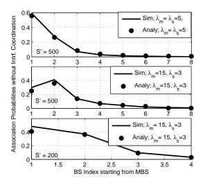
Fig. 3. Association probabilities of the NU with a reference MBS and S SBSs without interference coordination (for  $R_m = 300 \text{ m}$ , T = 100 m,  $\rho_m = \rho_s = 0$ ). BS indices  $[2, \dots, 4]$  represent the S SBSs within distance T.
