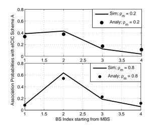
Fig. 4. Association probabilities of the NU with a reference MBS and S SBSs within distance T in eICIC scheme-A (for  $R_m = 300$  m, T = 100 m, S' = 200,  $\lambda_m = 15$ ,  $\lambda_s = 3$ ). BS indices  $[2, \dots, 4]$  represent the S SBSs within distance T.
