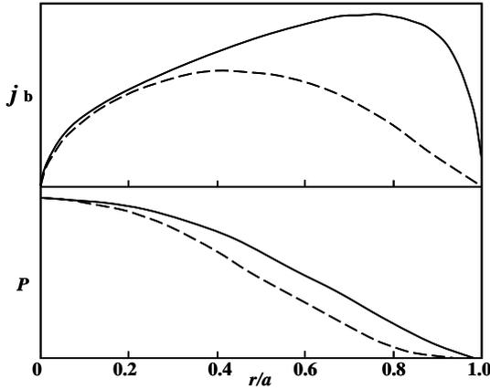
**Fig. 3** Typical bootstrap currents with a shift due to  $r/a$  where  $r$  is the radial direction of the Tokamak, and  $a$  is the inner radius of the Toroid This figure is reproduced from Wesson [3]
