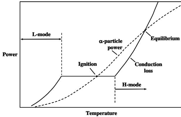
**Fig 5** Illustrating how increase in temperature can lead to the H mode region, in Tokamak physics where the designated equilibrium point, in Fig. 5 is a known way to balance conduction loss with alpha particle power, which is a known way to increase  $\tau_E$  i.e. Tokamak confinement of plasma time[2]
