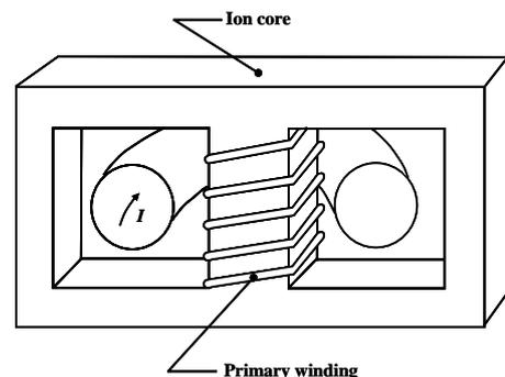
**Fig. 2** Flux change provided by a transformer core, in the simple current model first referred to in this paper. This figure is from Wesson [3]
