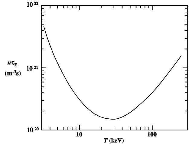
**Fig. 4** The value of  $n\tau_E$  required to obtain ignition, as a function of temperature. Figure reproduced from Wesson [3]
