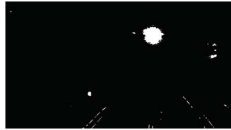
Fig. 7. False targets detected by the algorithm from low light reflections.
