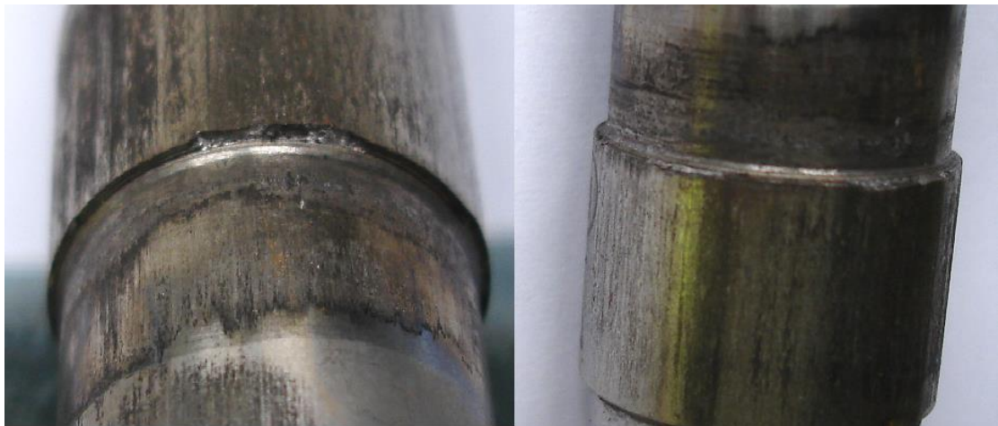
Fig. 4b. Enlarged view of two typical results of fusion ignition wherein the explosion gas pressure has broken pieces off the piston shoulders, in order to escape upwards.
