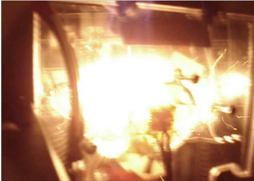
Fig.3b. Video camera snapshot of a typical fusion explosion, as viewed through a 12mm thick shatterproof polycarbonate window. The silicon photodiodes are mounted in the central region to view through a hole in the window, but are protected from flying debris by a stainless steel mesh. Some shaking of the whole enclosure and camera is always evident.
