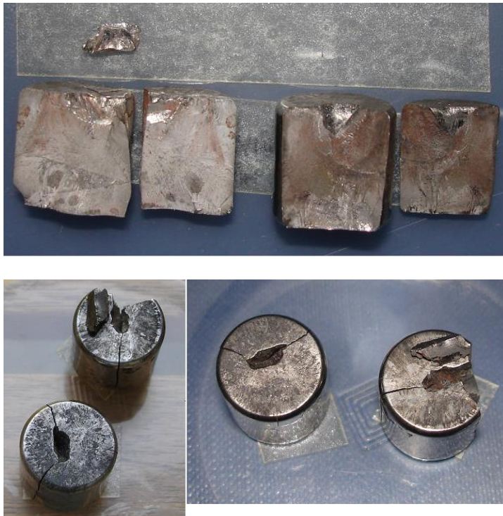
Fig 2b Two typical results of fusion ignition, wherein the local gas pressure has forced a wedge of steel downwards through the lower bearing, splitting it apart.
