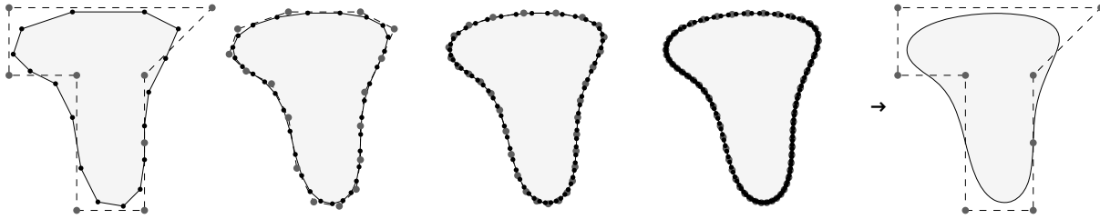
Figure: Several iterations of quartic B-spline subdivision applied to the T-shaped control point sequence with coordinates defined above. The area enclosed by the limit curve is \frac{74573}{20160} = 3.69905 \dots . The centroid is located at (\frac{490284845}{354370896}, \frac{212745589}{118123632}) . ■
