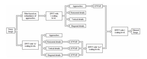
Fig. 1. Block diagram of the WDICWM algorithm.
