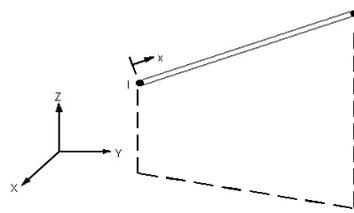
**Figure 8 Link8 Geometry**
