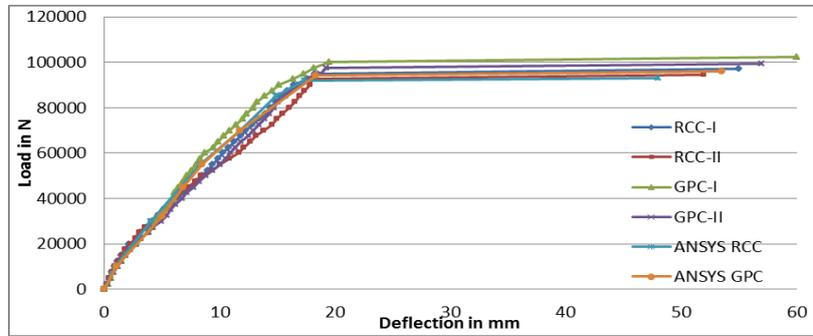
**Figure 9 Load-deflection Relationships for RCC and GPC Beams**
