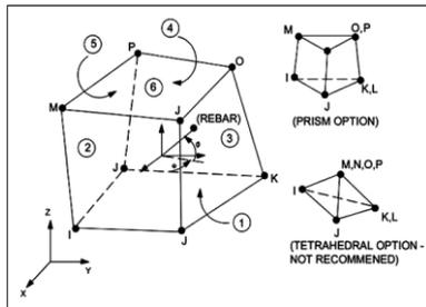
**Figure 7 Solid65 Geometry**
