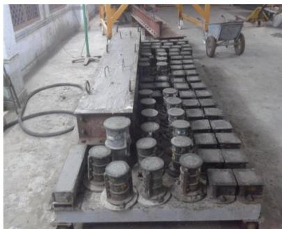
**Figure 3 Casting of Specimens**
