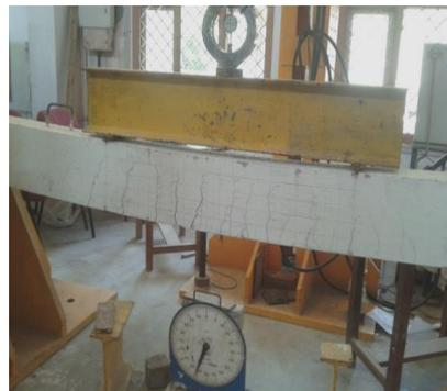
Figure 6 Crack Pattern of Beam
