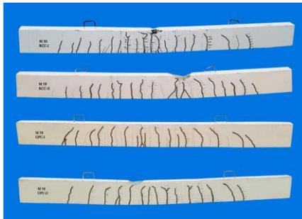
**Figure 10 Crack Pattern of Beams**
