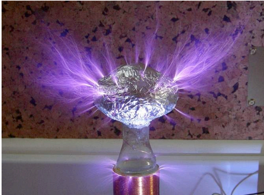
Figure 131. Corona discharge from a tesla coil, courtesy Robert Hunt .
