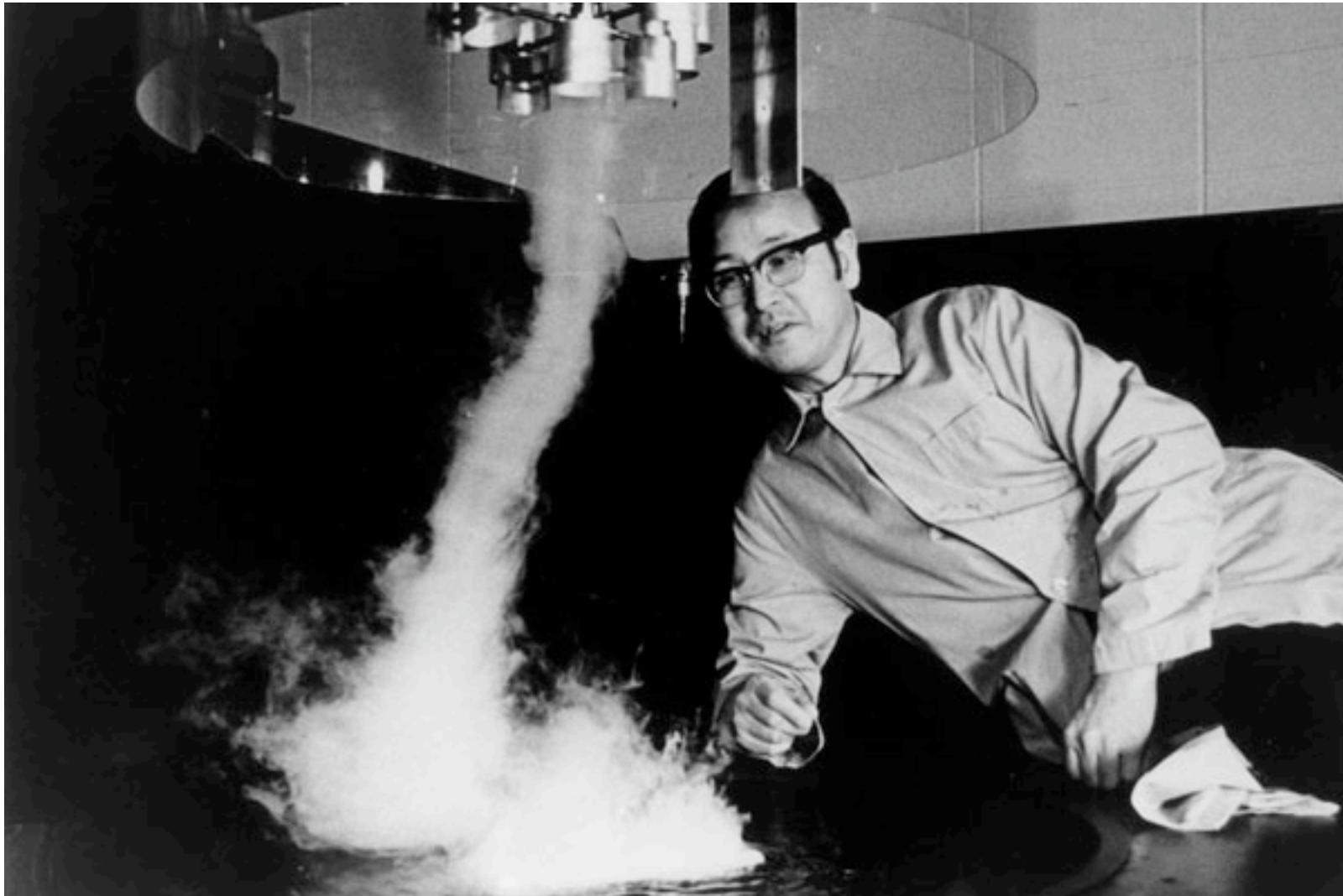
Figure 59. Ted Fujita's suction vortex experiment.
