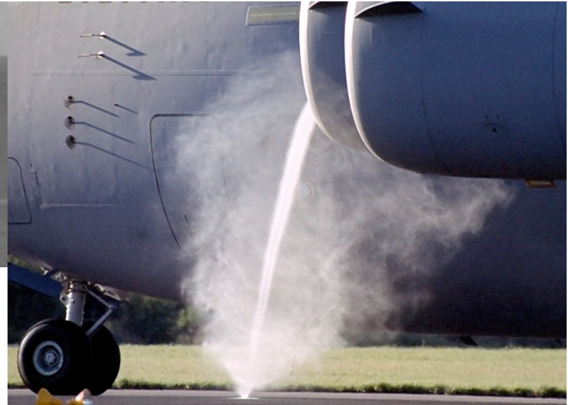
Figure 153. Suction vortex between a jet engine and the ground, courtesy Derek Ferguson .
