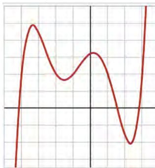
Graph of a polynomial of degree 5, with 3 real zeros (roots) and 4 critical points.
