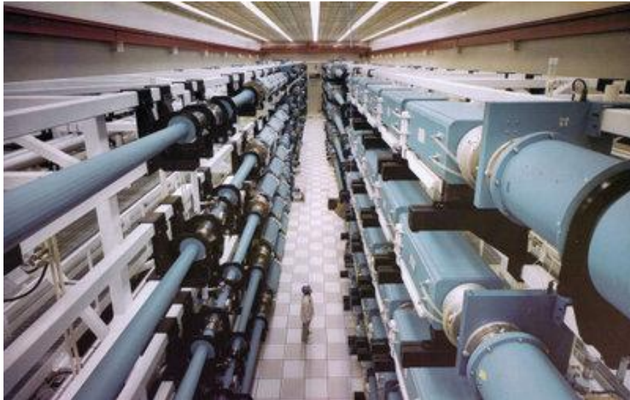
Fig. 2. Laser installation for NOVA inertial thermonuclear reactor. Look your attention in the man and gigantic size of laser installation for reactor. Cost is some billions of dollars.
