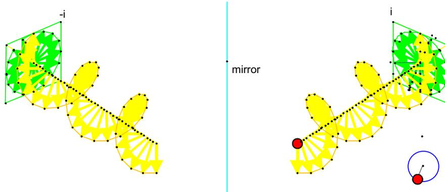
Figure 15: Right and left circular polarized waves  $\mathbf{q} = \mathbf{a} \exp(\mp I(\omega t - kx))$ .
