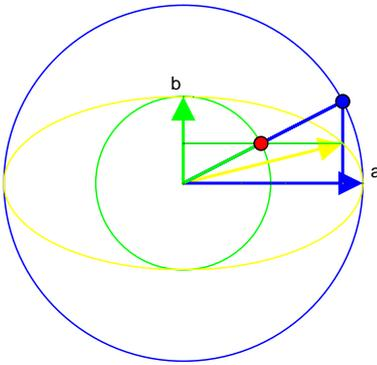
Figure 20: Description of ellipse by polar angle:  $\mathbf{r} = \mathbf{a} \cos \varphi + \mathbf{b} \sin \varphi$ .
