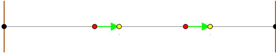
Figure 12: Symmetric longitudinal oscillations.
