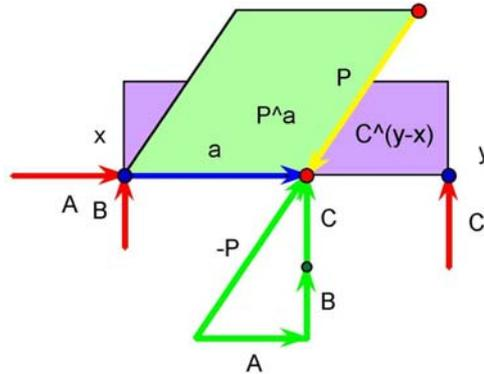
Figure 27: Beam with concentrated load.
