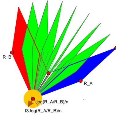
Figure 11: Rotation interpolation  $R_{inc} = \exp(\log(R_A/R_B)/n)$ .
