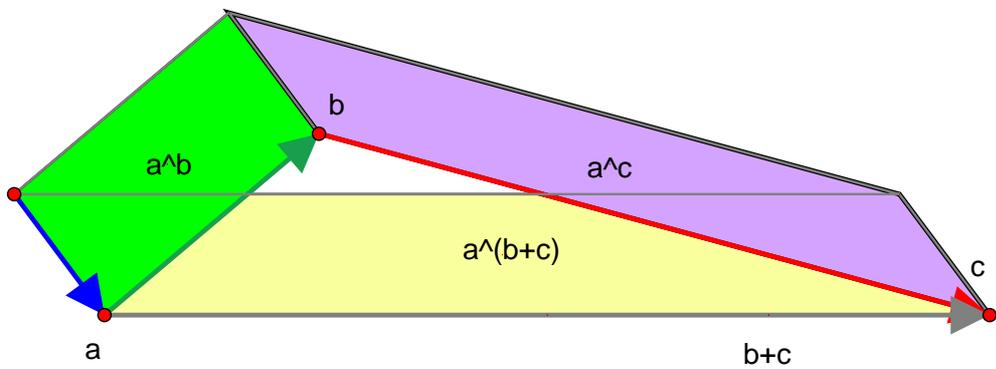
Figure 5: The outer product is distributive:  $\mathbf{a} \wedge (\mathbf{b} + \mathbf{c}) = \mathbf{a} \wedge \mathbf{b} + \mathbf{a} \wedge \mathbf{c}$ .
