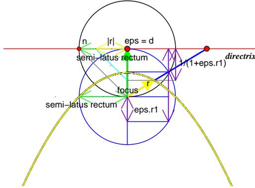
Figure 18: Semi-latus rectum generation of parabola:  $r = l/(1 + \epsilon \cdot \hat{\mathbf{r}})$ .
