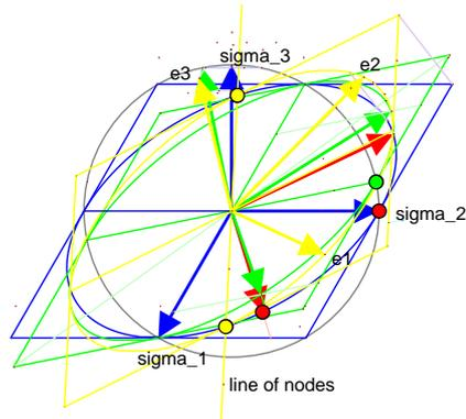
Figure 10: Euler angles of rotation  $R(\psi, \theta, \varphi)$ .
