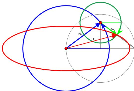
Figure 21: Description of ellipse by two coplanar circles:  $\mathbf{r} = \mathbf{a}_+ \exp(I_2 \Phi) + \mathbf{a}_- \exp(-I_2 \Phi)$ .
