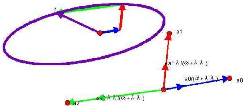
Figure 23: Ellipse as second order curve:  $\mathbf{r} = (\mathbf{a}_0 + \mathbf{a}_1\lambda + \mathbf{a}_2\lambda^2)/(\alpha + \lambda^2)$ ,  $\alpha > 0$ .
