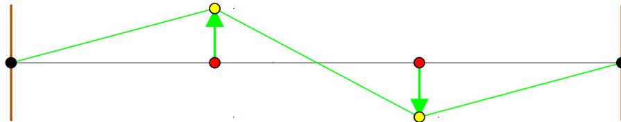
Figure 13: Antisymmetric transverse oscillations.
