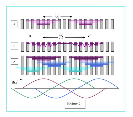
The flux density B(x) became time dependent B(x,t) if the DC current is replaced with a time dependent current i(t)
