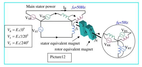
Pay attention to Picture 12.c The rotor rotate at 5Hz ( $f_R=5Hz$ ) and the stator equivalent magnet rotate at a different "speed" ( $f_S=50Hz$ ).
