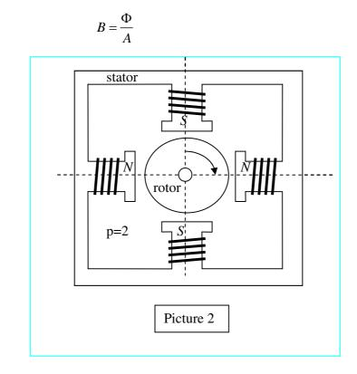
In rotating machines we have a moving part; the rotor and a static part; the stator. The rotor and stator have the same principles of operation.
