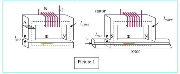
The magnetic reluctance of the iron core and the magnetic reluctance in air gap in picture 1 are;
