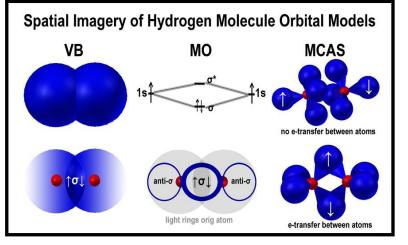
The bond strength of H-H (436 KJ/mole) is almost equal to that of O=O (497 KJ/mole). Thus, the two electrons provide significant coupling. The data tell us how much; what makes it happen is a different matter.
