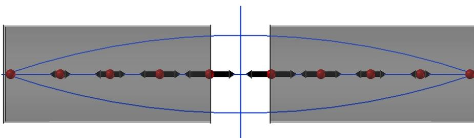
... that shows electrons oscillating backwards and forwards along the antenna and their
