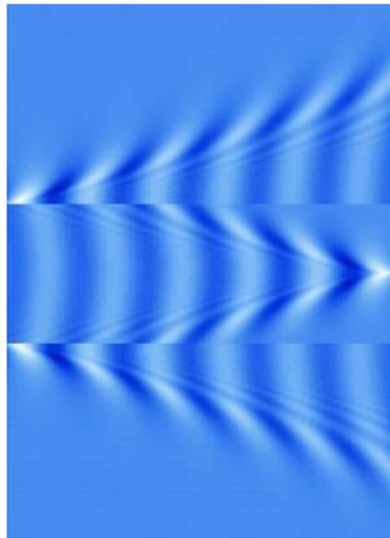
After a few oscillations a number of wavefronts moving in directions approximately perpendicular to the direction of the antenna are formed; the distance between two of wavefronts is the wavelength  $\lambda$  of the radio wave emitted:
