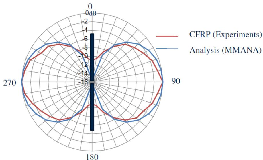
**Fig. 8.** Experimental and analytical two-dimensional radiation patterns of dipole antennas using the CFRP rectangular specimens. The analytical pattern was obtained using the antenna simulation software MMANA.
