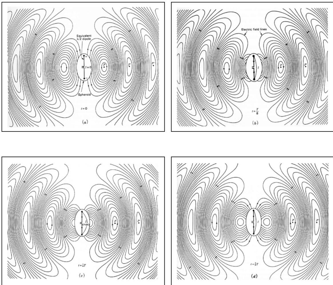
Five stages of radiation from a dipole antenna are shown in
