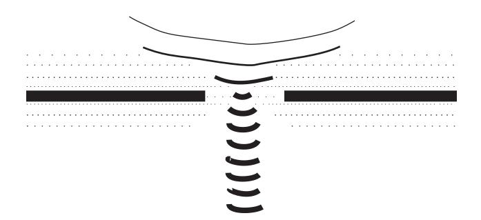
In the above diagram, the metal foil's EM field is represented by the surrounding dots. The waves become more concentrated (intense) as they meet with less resistance at the center of the hole. Sound waves and even surface water waves behave the same way.
