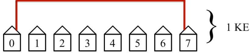
Figure 13. Only one key exchange is performed in this step. Host 1 through 6 are not allowed access to KLJN band thus they are in State 1. The seventh and the last step. This step is not efficient but only requires one KE since there is only one such pair of hosts.
