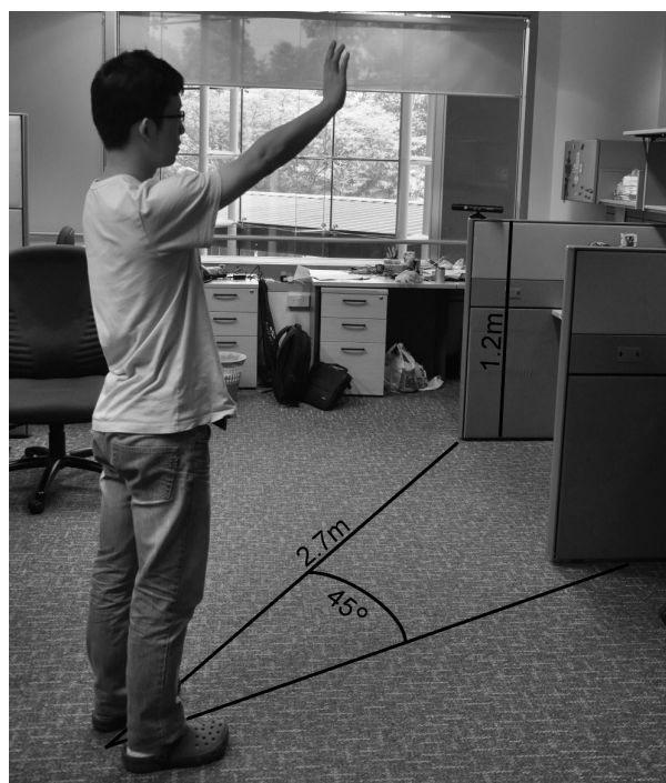
Figure 1. Experimental Setup: the user is facing the camera at angle of 45^\circ to the right of the sensor. Every arm movement is recorded at a fixed 2.7 m distance from the camera; where the camera is placed at height of 1.2 m above the floor.
