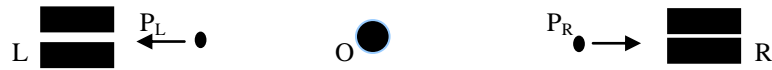
The experimental set up involves emitting of two spin \frac{1}{2} particles P_L and P_R having opposite spin states from a system at O. Two detectors L and R kept at a large distance from each other measures the spin state of the particles at the same instant.
