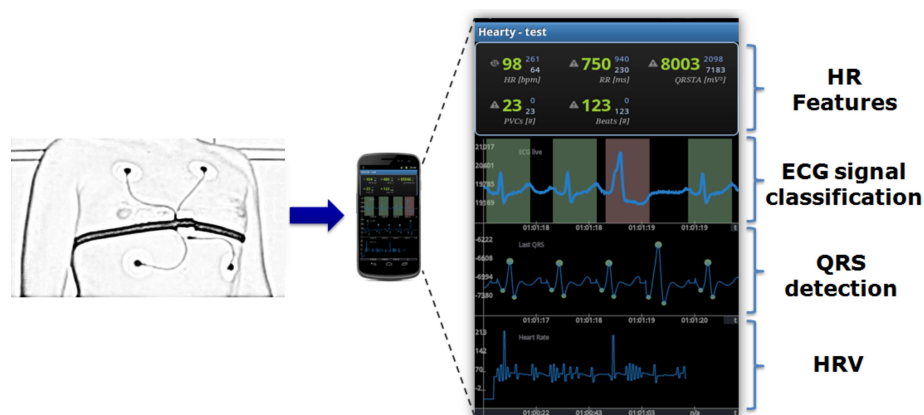
Figure 4. Screenshot showing the main interface of the 'Hearty' application implemented by Gradl et al. (2012) [8]. From top to bottom: Panel showing various clinically relevant parameters that are automatically detected including heart rate (HR) and RR interval; Panel showing the detected ECG signal, which is wirelessly streamed to the application; Panel showing the QRS detection with filled circle markers for the Q, R and S waves; Panel showing the detected beat-to-beat heart rate.
