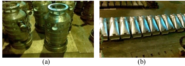
Fig. 3. Gas turbine MW 701 D combustor sections (a) Combustor basket, (b) Transition piece.
