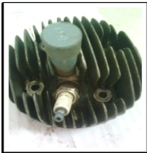
Fig.3: Metal plug & spark plug in position
