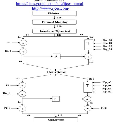
Fig. 2 Modified blowfish algorithm
