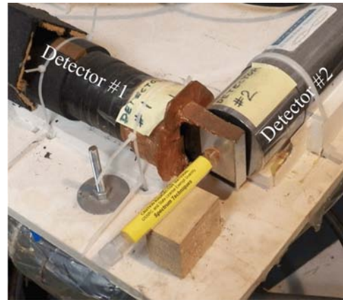
Fig. 2 Two gamma-ray detectors in tandem geometry; a demonstrator unit. (50) Detector #1 was used with other components for data shown.
